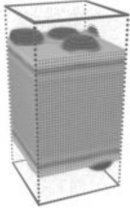
Fig. 11. 3D sample at off-critical composition. Initial concentrations are as in Figure 6, kT/\epsilon_{AA} = 0.75 , and t = 20\,400\omega_0^{-1} .
